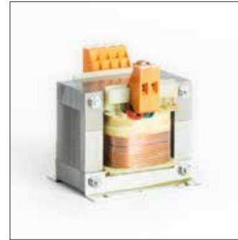
Through their additional  $\pm 5\%$  tapings, control transformers equalise mains undervoltages and overvoltages and are able to suppress short circuit in case of malfunction to permit auxiliary circuits to function unearthed. A control transformer has two separate coils. Version sizes range from single-phased up to 25 kVA and multi-phased up to 40 kVA. Coil types are available in solder plug, clamp and bracket versions.
