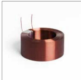
Air-core coils are inductive components without a ferromagnetic core and therefore have relatively low inductance. The magnetisation curve is linear. Air-core coils feature no magnetic saturation compared to coils with magnetic cores. Without a core, magnetic paths cannot be guided resulting in a high level of magnetic flux leakage.
