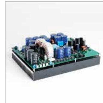
We develop and manufacture high quality charge controllers which comply to all current standards and use the latest power electronics, microprocessors and a special charger IC. To control charging, we use, for example, parameters which determine temperature, voltage, capacitance, time, and charging current.
