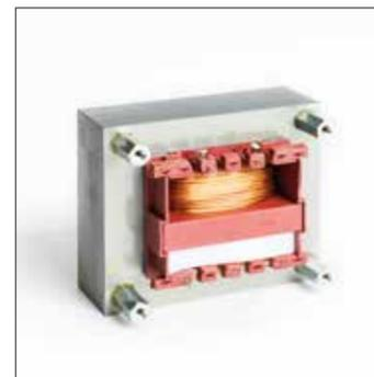
Safety transformers output secondary low voltages for SEL and PELV circuits. A safety transformer has 2 separate coils which may not hold in excess of 50 VAC and 120 VDC when idling. Version sizes range from single-phase to 10 kVA and multi-phase up to 16 kVA. Coil types are available in solder plug, clamp and bracket versions.
