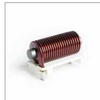
Output chokes are connected in front of inverters to minimise their negative effects. Voltage spikes from in-line motors are reduced to increase motor service life by diminishing insulation loads.
