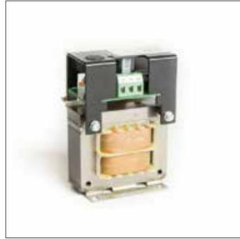
Mains transformers have the task of transforming input voltages to the required output voltages. A mains transformer has two separate coils. Version sizes range from single-phase to 1 kVA and multi-phase up to 5 kVA. Coil types are available in solder plug, clamp and bracket versions.
