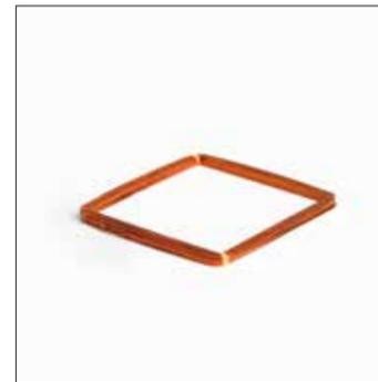
A special version of enamelled wire is self-bond enamelled wire. Its adhesive properties are activated thermally or by a solvent. After activation, the individual windings bond into a self-sustaining coil. The use of self-bond enamelled wire gives a range of cost and manufacturing benefits due to the savings made on coil forms, adhesive tape, casting compounds and impregnation. We are able to manufacture these coils in a range of different sizes and shapes.
